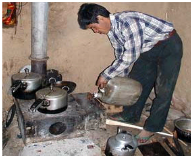
Plate 7: The most modern smokeless stove – it has 3 hot plates, a 9 litre water container and a slot for charring roti.
